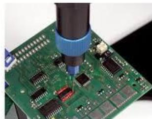
THE CF ECO SERIES VOLUMETRIC VALVES ARE A PURELY VOLUMETRIC DISPENSING SYSTEM THAT APPLIES THE SMALLEST AMOUNTS OF SINGLE-COMPONENT FLUIDS FOR HIGH-PRECISION DISPENSING TECHNOLOGY.
